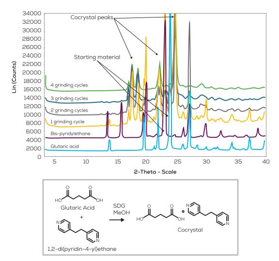
Figure 9: XRD data from the manual SDG method demonstrates that after four grinding cycles, cocrystal formation was complete.
