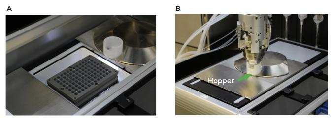
Figure 6: (A) The deck of the Big Kahuna with the crystallizer assembly in the on-deck balance. (B) The solid dispensing arm with hopper containing powder to be dispensed.
