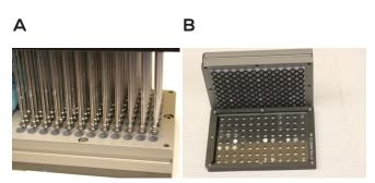
Figure 8: (A) Steel ball removal. (B) Opening the crystallizer assembly.
