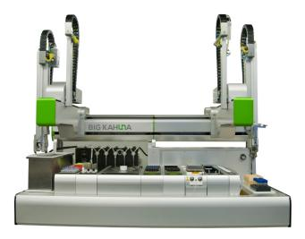
Figure 3: The Big Kahuna system is a fully configurable, automated system for preparing, processing and testing chemically complex samples and mixtures. The Big Kahuna system can be used to automate SDG cocrystal generation using the system's liquid and solid dispensing, vortexing and weighing capabilities.
