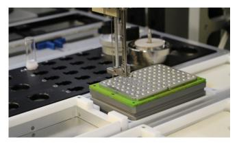
Figure 7: The Big Kahuna automatically dispenses the required amount of solvent to the plate.
