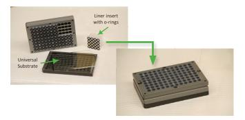
Figure 4: The crystallizer assembly is composed of a 96-well plate, a glass or quartz plate (universal substrate) and disposable liner inserts. The steel balls and the compounds will be deposited in the liner insert. O-rings at the bottom of the insert will ensure that the material in each well remains isolated. The cocrystals will be formed on the universal substrate, which can be removed for analytical testing without further manipulation of the cocrystals.
